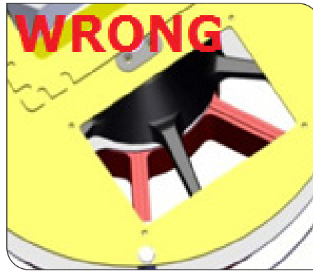
Illustration 29: Correct and wrong positioning of rotor, seen from above
